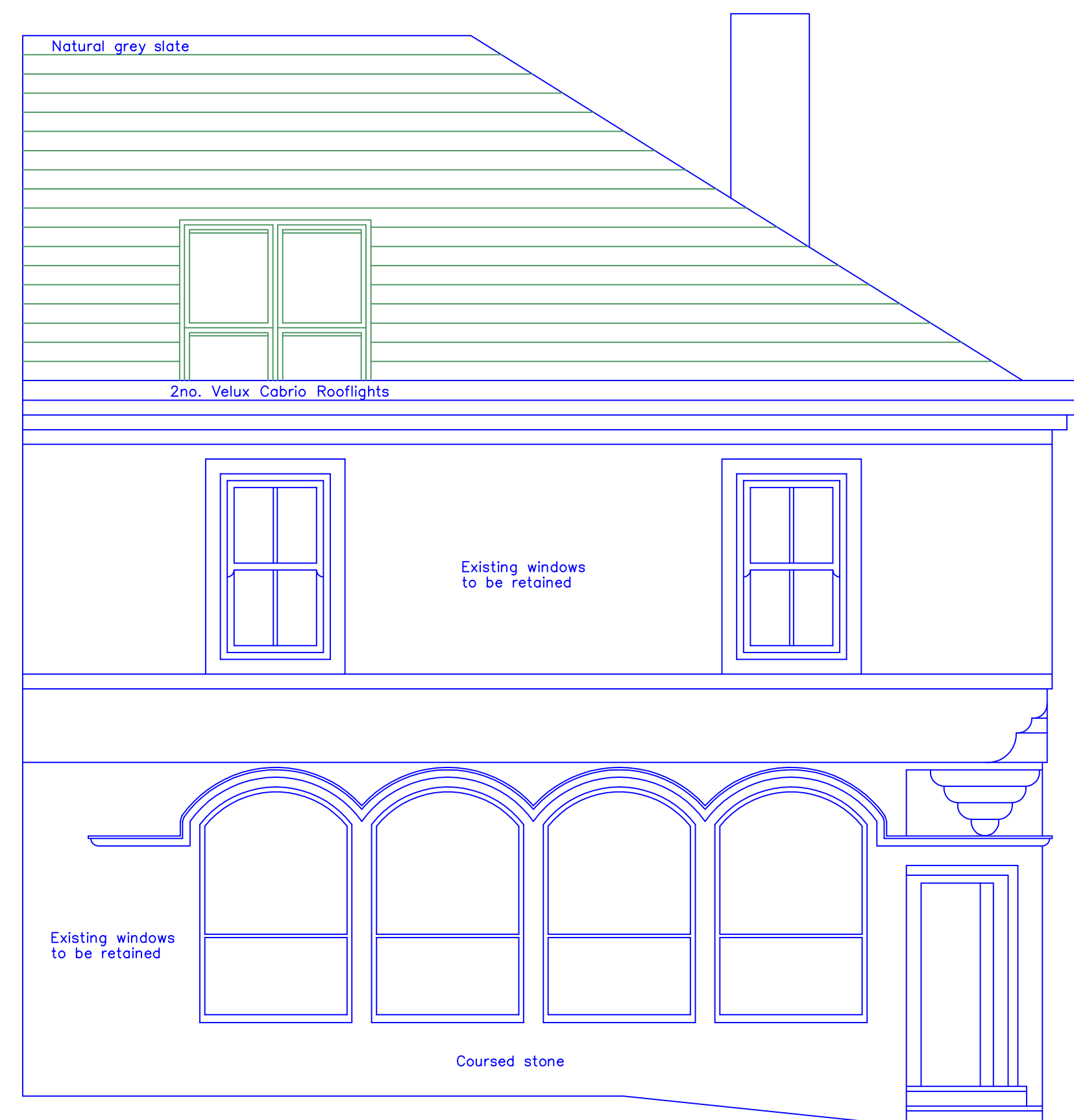
PROPOSED SOUTH ELEVATION along Bridge Street
